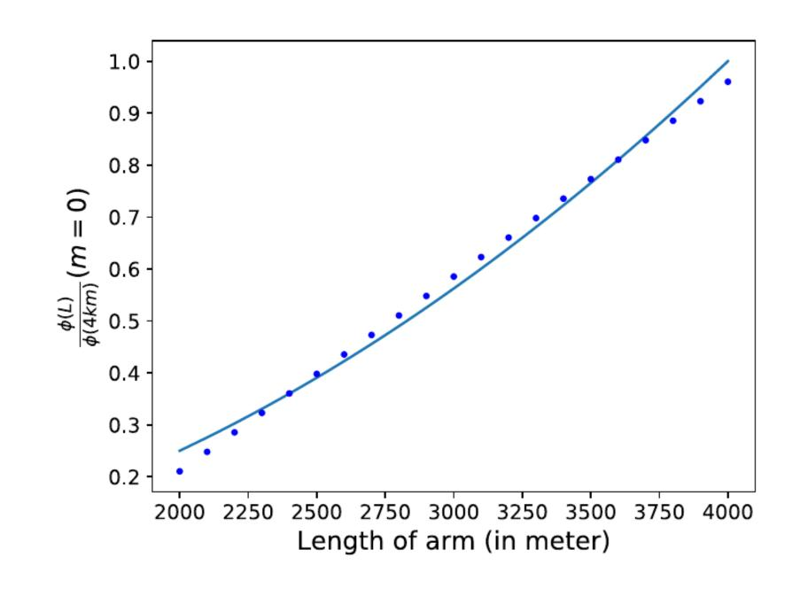
Phase difference between two arms of interferometer clearly deviates from linear nature for GW beams:
